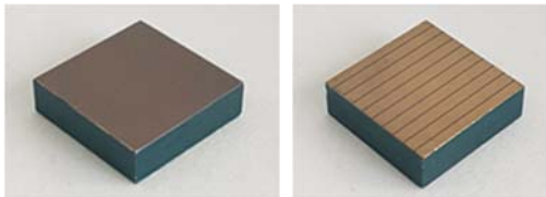
Figure 4. One of Redlen CZT used for 3D spectro-imager module; (left) anode side (48 strips) and (right) cathode one (10 cathode strips).
